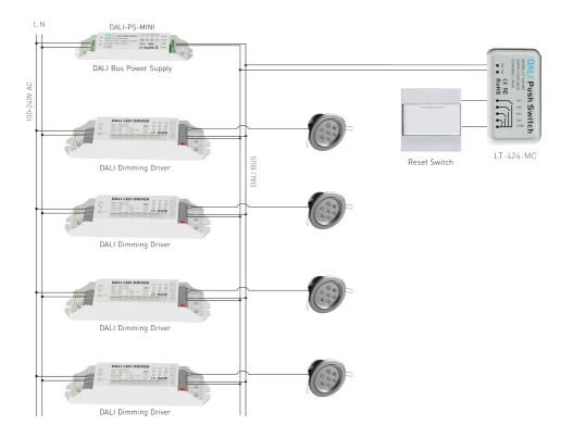
Installation: 1. Disconnect the power supply of all devices on the DALI bus before installing.
